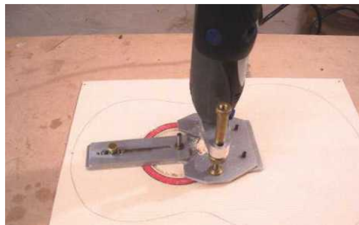
STEP 7. Removing waste wood from the soundhole
